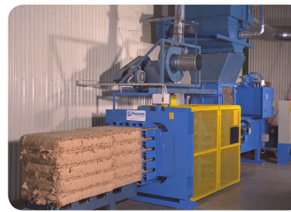
Compaction unit (baler)
